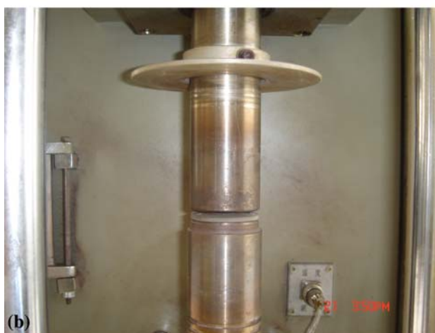
Fig. 1 System of wearing test (a) pin-disc wearing counterpart; (b) testing contact equipment
